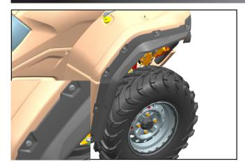
This picture shows the assembled state of the right front extended fender.
