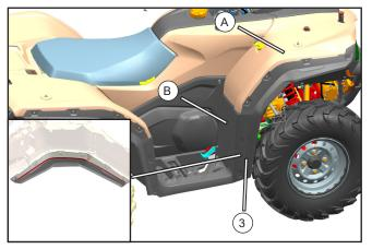
// Align the two red parts of the right front extended fender (3) to the front fender (A) and the right foot pedal (B) as shown in the inset image, then mark the 6 holes on the right front extended fender with a marker.
