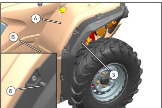
Secure the right front extended fender (3) with plastic clips (6).
