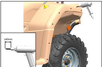
Use the electric drill to drill the marked 6 holes in turn.
